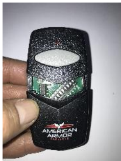
Slide dip switch cover down sets switch code
